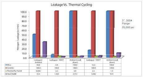
Laboratory testing demonstrates the long term, high temperature stability of the THERMa-PUR™ material compared to existing materials
