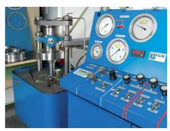
To ensure conistent high quality valves all components are subjected to stringent testing running in parallel with all stages of production.
