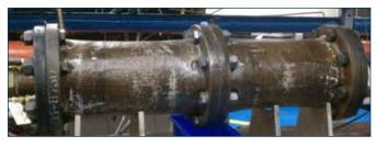
Style 3504 GYLON® STRESS SAVER® showed no signs of leakage when installed between smooth, flat face FRP flanges – the flange assembly was subjected to over 3,000 thermal cycles without a re-torque.
