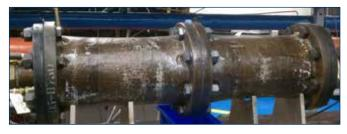
STRESS SAVER® GYLON® 3504 showed no signs of leakage when installed between smooth, flat face FRP flanges – the flange assembly was subjected to over 3,000 thermal cycles without a re-torque.
