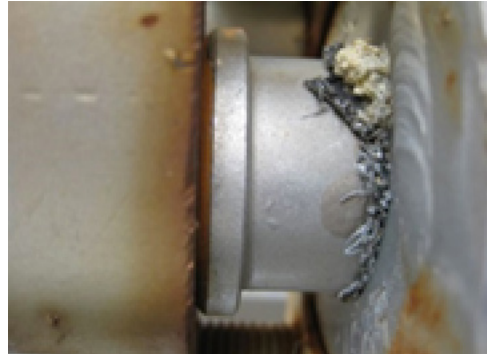
Figure 2: Improper installation: packing out stuffing box
