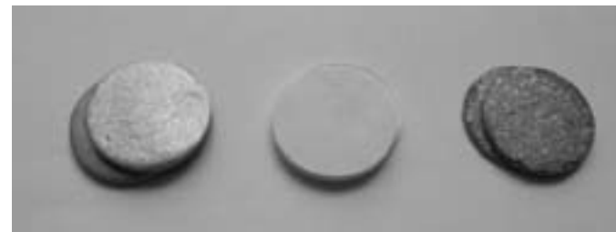
Fig. 1 Typical compressible gaskets (from left) mica-, talc- and vermiculite-based materials
