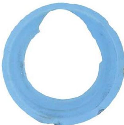
Figure 3. Effects of erosion on a PTFE gasket
