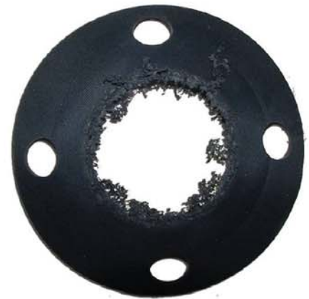
Figure 1. Effects of overcompression on a rubber gasket in a raised-face flange
