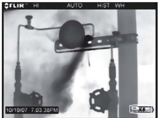
Figure 2. An alternative to Method 21 is optical gas imaging using handheld, forward-looking infrared cameras, the optics and analyzers of which are tuned to "see" fugitive emissions. (Photo courtesy of Sage Environmental Consulting)
