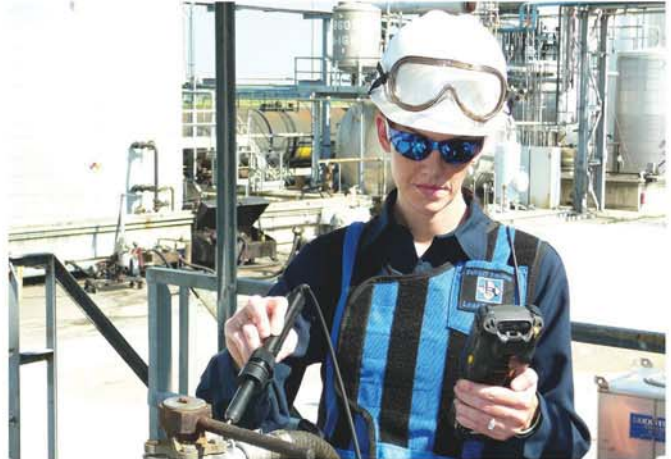
Figure 1. Method 21 requires each regulated component to be monitored for fugitive emissions at monthly, quarterly or annual intervals, using organic or toxic vapor analyzers. In a typical chemical plant or oil refinery, this could involve tens of thousands of points. (Photo courtesy of TEAM® Industrial Services)
