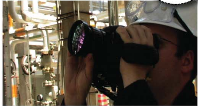
Figure 2. An alternative to Method 21 is optical gas imaging using handheld, forward-looking infrared cameras, the optics and analyzers of which are tuned to "see" fugitive emissions. (Photo courtesy of Sage Environmental Consulting)
