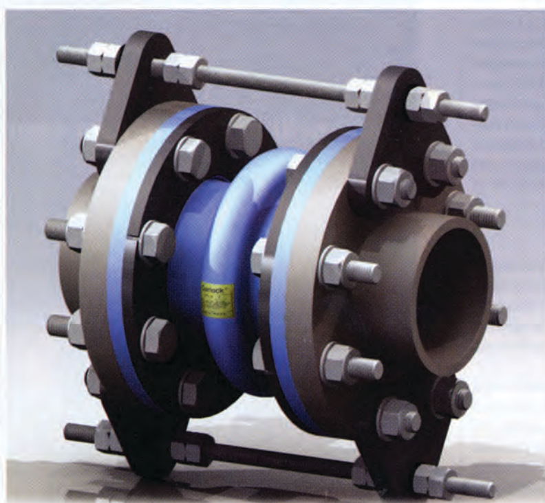
Figure 1: This spool-type expansion joint with control units features a single arch to accommodate both angular and linear pipe movement. Courtesy: Garlock Sealing Technologies
