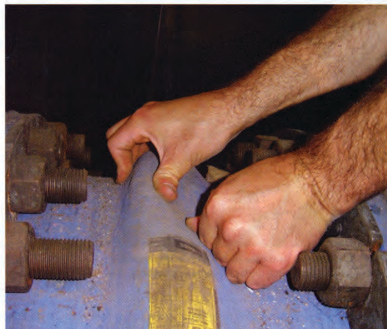
Figure 2: A soft arch that can be pressed into indicates the tube inside the expansion joint has been compromised, allowing aggressive media to come into contact with the body and cover. Courtesy: Garlock Sealing Technologies
