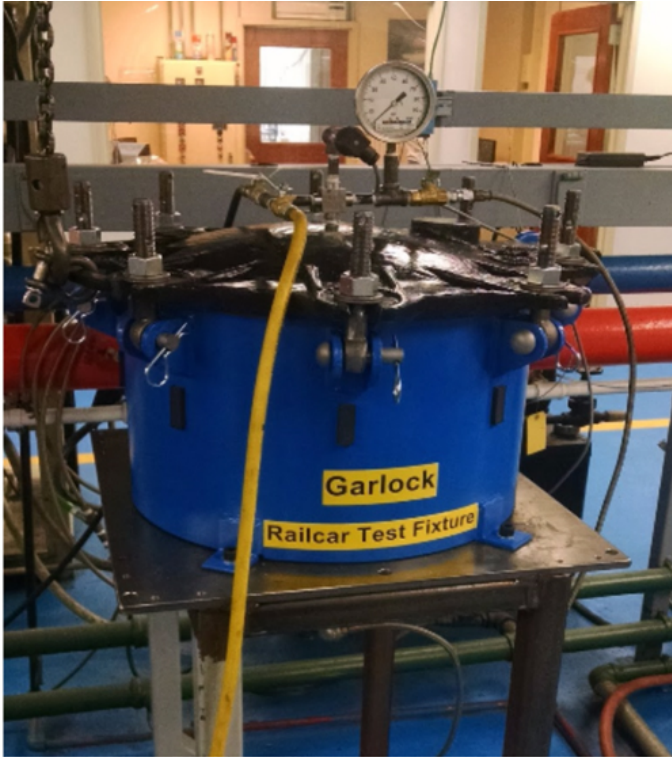
Fig. 3 AAR-1 Rail test fixture
